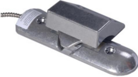
This roller shutter contact can be used in most security systems up to and including grade 1 & 2 as specified in EN50131-1:2006 and is compliant with EN50131-2-6:2008 and environmental class III. It operates as a normally closed circuit going open when the magnet housing is moved away from the contact housing. This contact can be used on roller shutter doors to detect the unauthorised entry of an intruder. The contact is sealed to prevent access to the inside.
