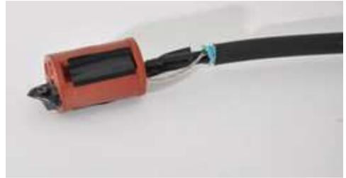
**3) Use the foil to shield the end connection.**
